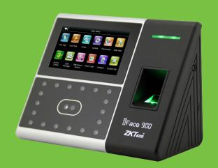
ZKTeco has released the iFace900 Multi-Biometric T&A and Access Control Terminal which supports 3,000 face templates, 4,000 fingerprint templates and 10,000 cards. It is equipped with ZKTeco latest hardware plat-form and algorithm, which provide clients with a brand new UI and user-friendly operating interface, bringing them a smooth using experience. With the advanced face algorithm and multi-biometric verification technology, the terminal's security level of verification is greatly enhanced.
